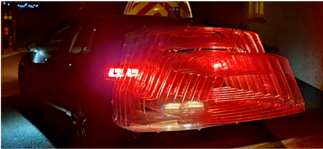
Figure 9: Inflatable double-cavity device. Reproduced from Ref. [9] under the Creative Commons Attribution (CC BY) license.
